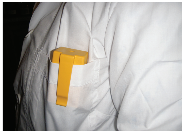
Fig. 3. Personal monitor Radman XT was worn on the body, attached to clothing with a plastic clip.
