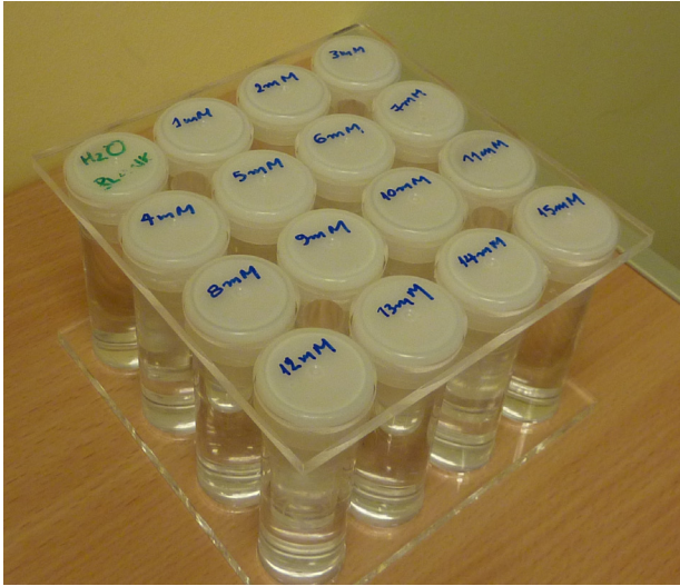
Fig. 1. Fifteen 30 ml polycarbonate cylindrical vials containing Gd-doped deionised water solutions with Gd concentration ranging from 1 mM to 15 mM and one 30 ml vial of clear deionised water (upper left) were mounted in a Plexiglas case.
