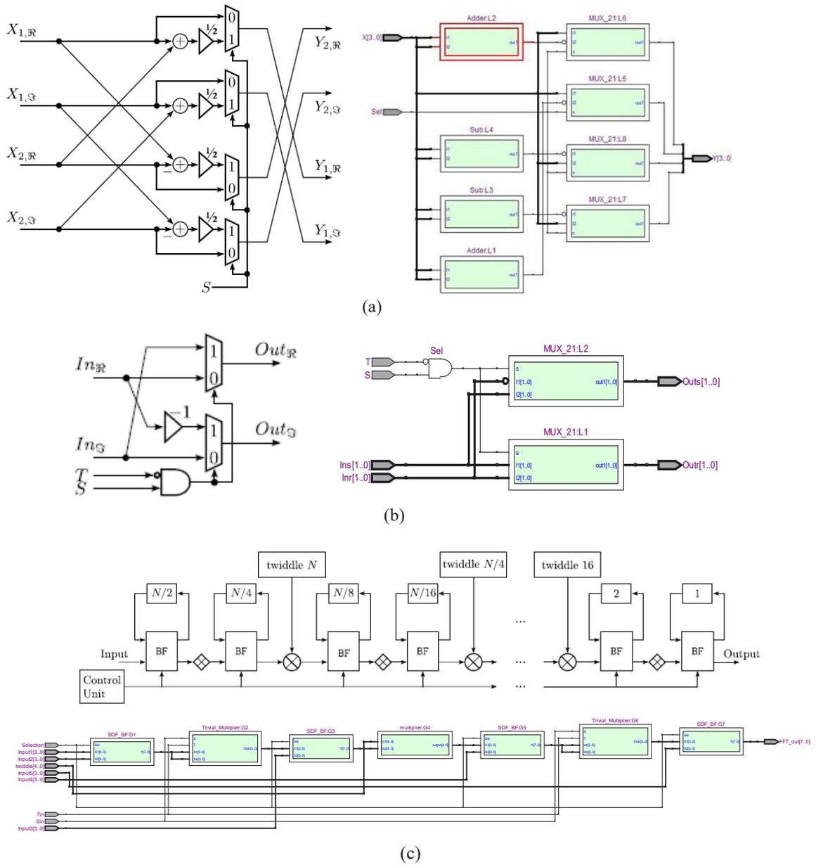
Figure 3 The Circuit and RTL view of (a) SDF-BF (b) Trivial Multiplier (c) N-point radix-22 SDF pipeline FFT core
