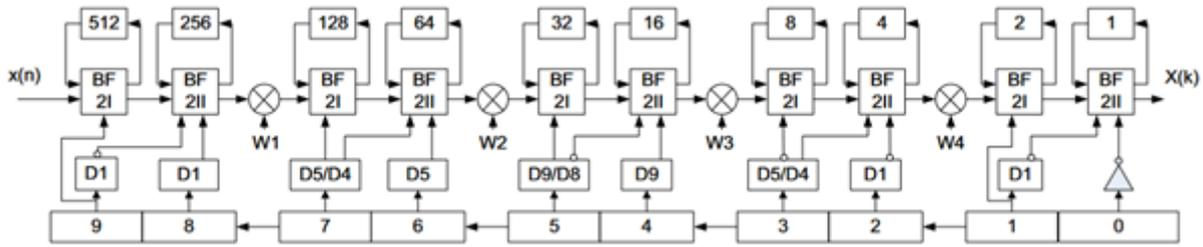
Figure.2. N-point radix-22 SDF pipeline FFT core
